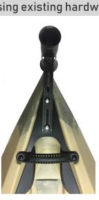
2. Mount Anchor Wizard chute to Bracket with provided hardware
