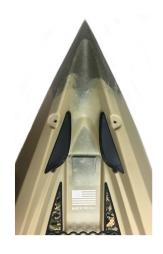
3. Reinstall bow handle over bracket reusing existing hardware
