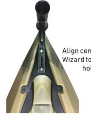
Align center hold on Anchor Wizard to the forward-most hole on bracket
