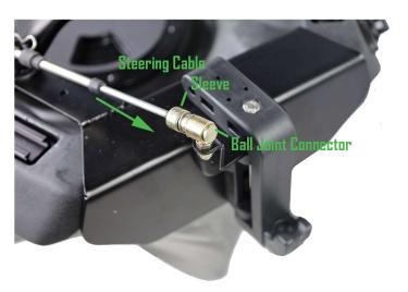
b. Place steering cable in bracket clamp and secure with cotter pin.
