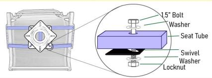
5. Install swivel to seat base using hardware from this pack.
