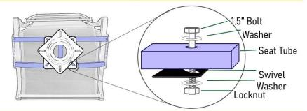
5. Install swivel to seat base using hardware from this pack. (Use two 7/16" wrenches or adjustable wrenches to tighten)
