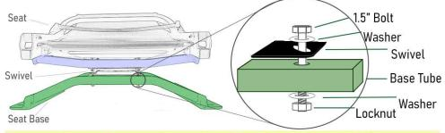
6. Install seat on boat using Mighty Bolts + Mighty Knobs
