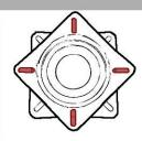
3. Secure swivel to seat frame using 1.5" bolts. (Use two 7/16" wrenches or adjustable wrenches to tighten)
