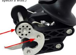
c. Remove remaining Lock Nut securing top Swing Arm, then remove Swing Arm.
