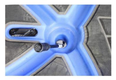
c, Feed transducer cord and handle through Mount Cap.
