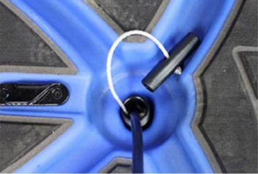
d. Twist Mount Cap to tighten and secure in place, pull handle tight and secure on clam cleat.
