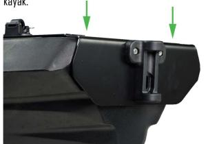
b. Insert hex bolt from the outside, and secure with washers and Tri-knob.
