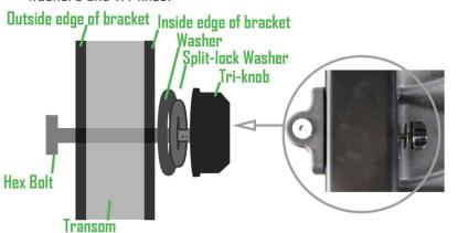
c. Attach swing arm to transom bracket. Insert 5-1/2" Hex Bolt from the top (making sure it seats into hex-shaped recess) and secure with nylon thumb screw from the bottom.
